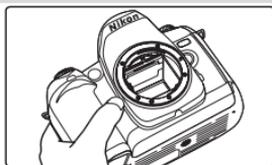
**5** Turn the camera off. The mirror will return to the down position and the shutter curtain will close. Replace the lens or body cap and disconnect the AC adapter.
