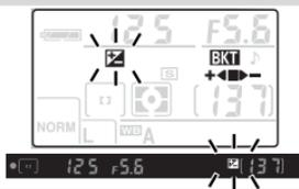
**4** Take a series of three photographs. The first photograph will be taken at optimal exposure, the second will be underexposed by the selected exposure increment, and the third overexposed by the same amount. A segment will disappear from the bracketing progress indicator after each shot. Repeat Steps 3–4 to record additional bracketing sequences.
