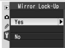
**3** Press the shutter-release button all the way down. The mirror will be raised and the shutter curtain will open, revealing the low-pass filter, and a row of dashes will blink in the control panel.
