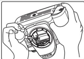
**3** Turn the camera off. The mirror will return to the down position and the shutter curtain will close. Replace the lens or body cap.
